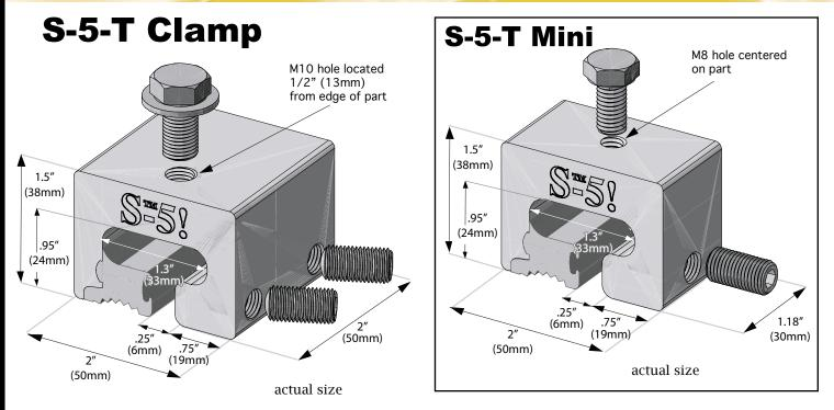
The S-5-T and S-5-T Mini clamps are each furnished with the hardware shown above. Each box also includes a bit tip for tightening setscrews using an electric screw gun. A structural aluminum attachment clamp, the S-5-T is compatible with most common metal roofing materials excluding copper. All included hardware is stainless steel. Please visit www.S-5.com for more information including CAD details, metallurgical compatibilities and specifications.
