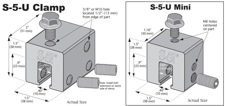
The S-5-U and S-5-U Mini clamps are each furnished with the hardware shown above. Each box also includes a bit tip for tightening setscrews using an electric screw gun. A structural aluminum attachment clamp, the S-5-U is compatible with most common metal roofing materials excluding copper. All included hardware is stainless steel. Please visit **www.S-5.com** for more information including CAD details, metallurgical compatibilities and specifications.
