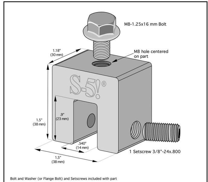
The S-5-S and S-5-S Mini clamps are each furnished with the hardware shown above. Each box also includes a bit tip for tightening setscrews using an electric screw gun. A structural aluminum attachment clamp, the S-5-S is compatible with most common metal roofing materials excluding copper. All included hardware is stainless steel. Please visit [www.S-5.com](http://www.S-5.com) for more information including CAD details, metallurgical compatibilities and specifications.
