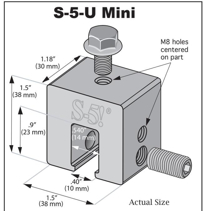
The S-5-U and S-5-U Mini clamps are each furnished with the hardware shown above. Each box also includes a bit tip for tightening setscrews using an electric screw gun. A structural aluminum attachment clamp, the S-5-U is compatible with most common metal roofing materials excluding copper. All included hardware is stainless steel. Please visit [www.S-5.com](http://www.S-5.com) for more information including CAD details, metallurgical compatibilities and specifications.
