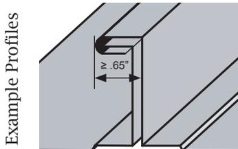
For horizontal seams under .65" do not use this clamp. Visit [www.S-5.com](http://www.S-5.com) for more detailed information and proper clamp to use.
