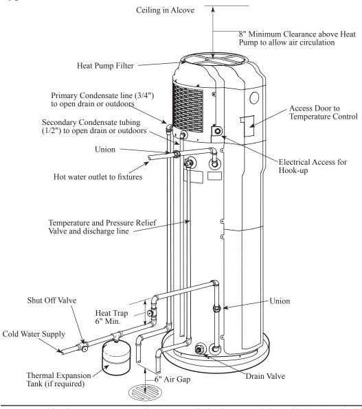
A new combination temperature and pressure relief valve, complying with the Standard for Relief Valves and Automatic Gas Shut-Off Devices for Hot Water Supply Systems, ANSI Z21.22/CSA 4.4, is installed in the opening provided. No valve of any type should be installed between the relief valve and the tank. Local codes shall govern the installation of relief valves.
